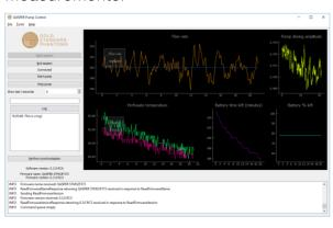
At the heart of the QASPER phantom is an MRI compatible pump that delivers liquid at a known flow rate. Its flow rate can be monitored, controlled and recorded in real time by software, providing complete assurance during image acquisition that the phantom is operating as intended.
